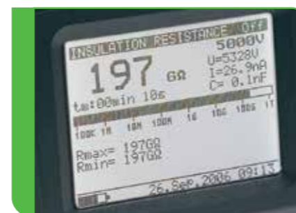
Large custom LCD dot matrix display with bar graph and backlight.
