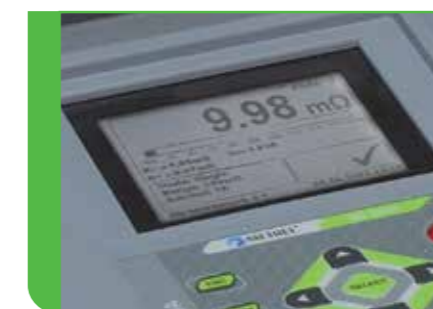
Large analogue / digital LCD with backlight
