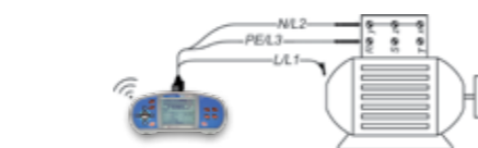
Test circuit for continuous resistance measurement
