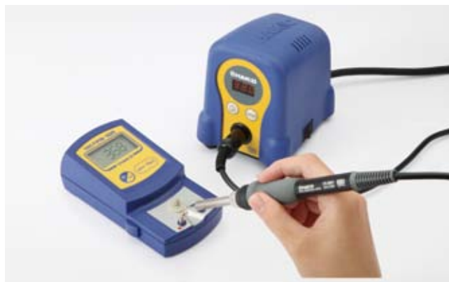
Measuring the tip temperature with a tip thermometer (HAKKO FG-100)
